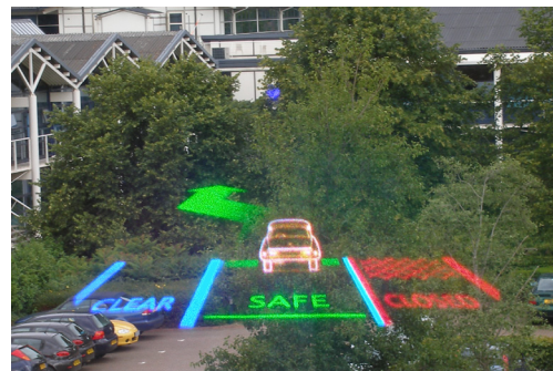
Figure 7 - Sample image demonstrating the performance of LBO's full-colour rear-view virtual image display.
