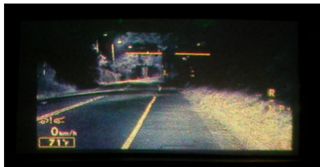
Figure 8 – Example of night vision [21] virtual image at WVGA resolution formed using LBO's holographic laser HUD.
