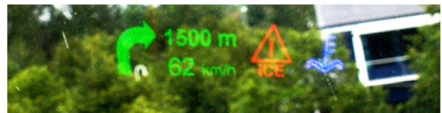
Figure 7 – Example symbology-type imagery formed using LBO's holographic laser HUD, captured in daylight.
